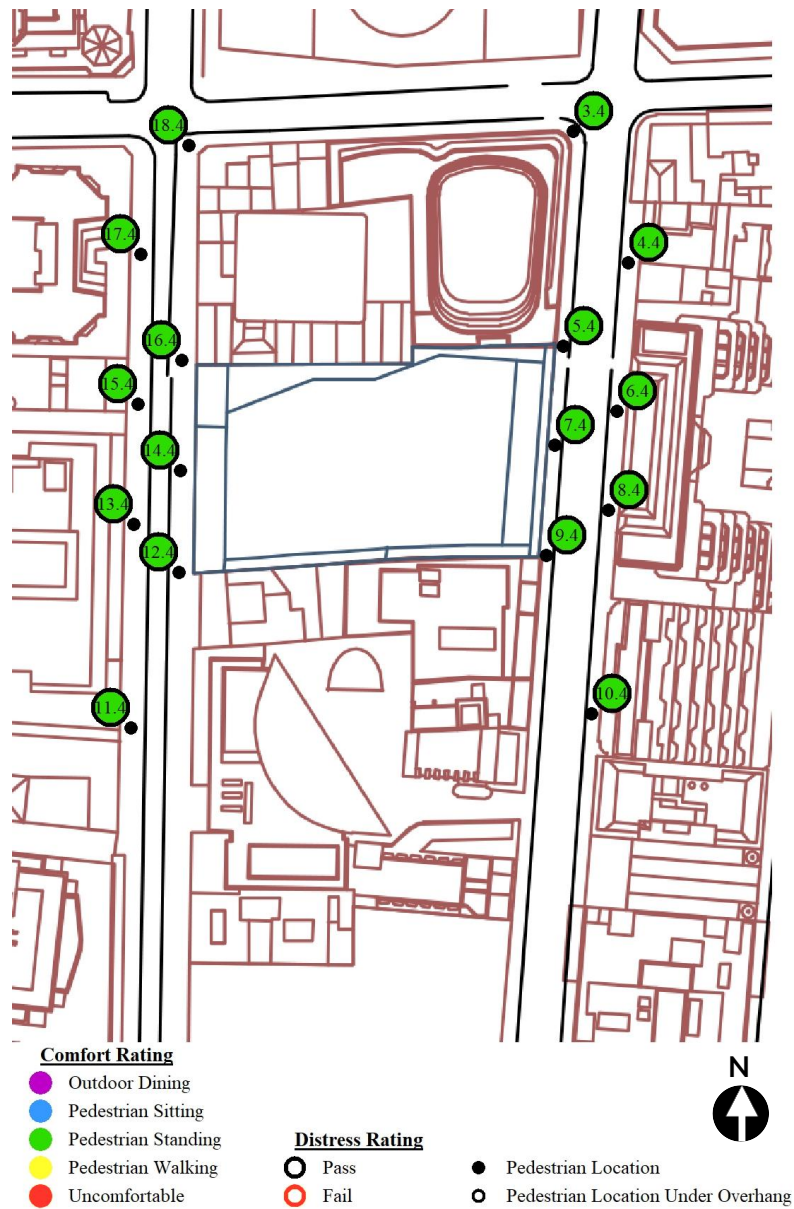
Figure 11: Pedestrian wind speed measurement locations with comfort/safety ratings. Ground – Configuration D: Proposed all office
