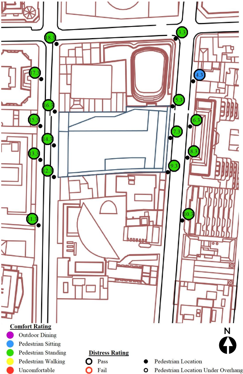
Figure 10: Pedestrian wind speed measurement locations with comfort/safety ratings. Ground – Configuration C: Proposed mixed-use
